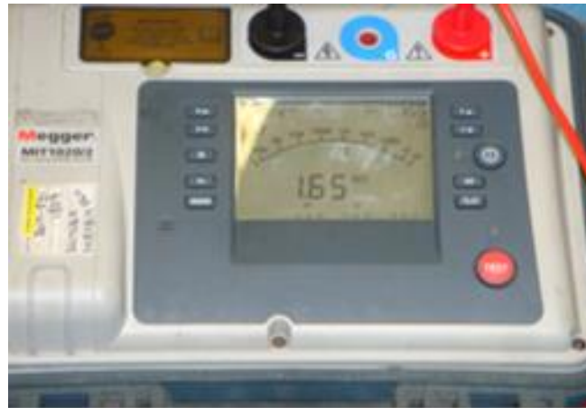
Figura 2.22 Megger MIT1020/2, Insulation Tester 20TΩ CAT IV 600 V 10kV 5mA
