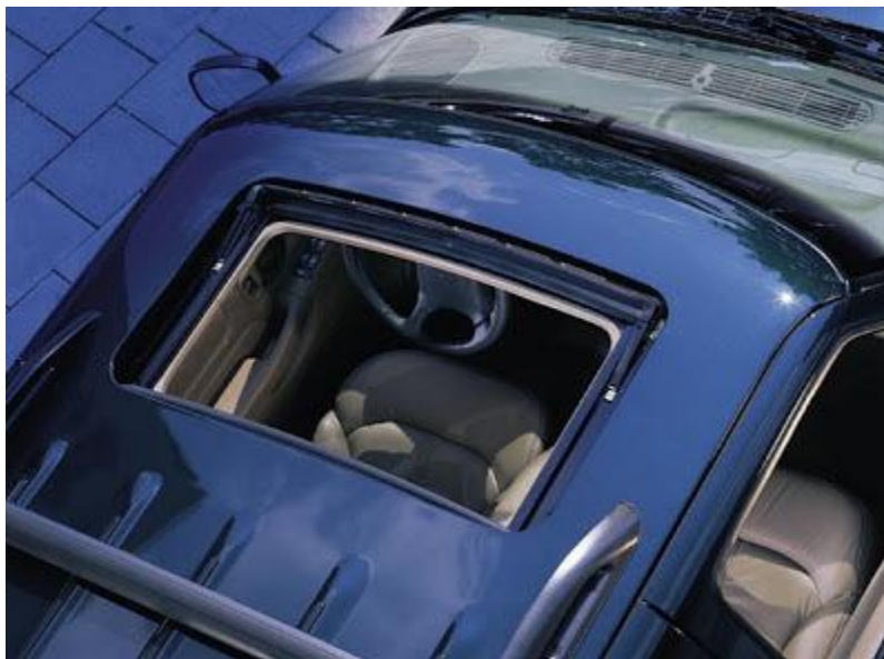
Figura 8 Techo solar tipo In built.
