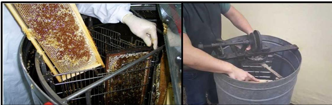
Figura 12 extractor centrifugo
