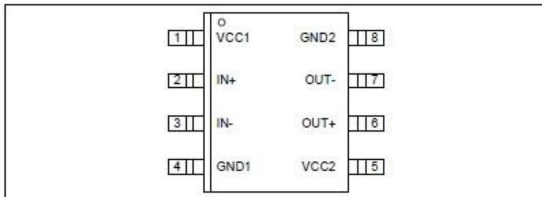
Figure 3 PG-D80-8-51 (top view)
