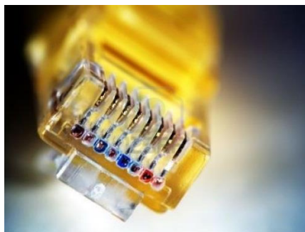
fig.2.12 Cable Ethernet RJ 45
