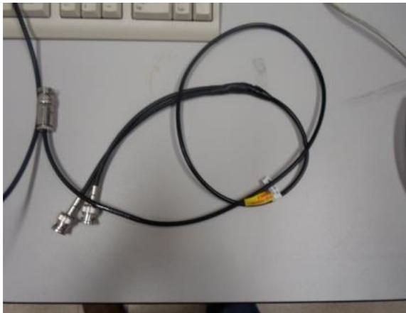
Fig.4.9 Cable adaptado de triaxial a coaxial
