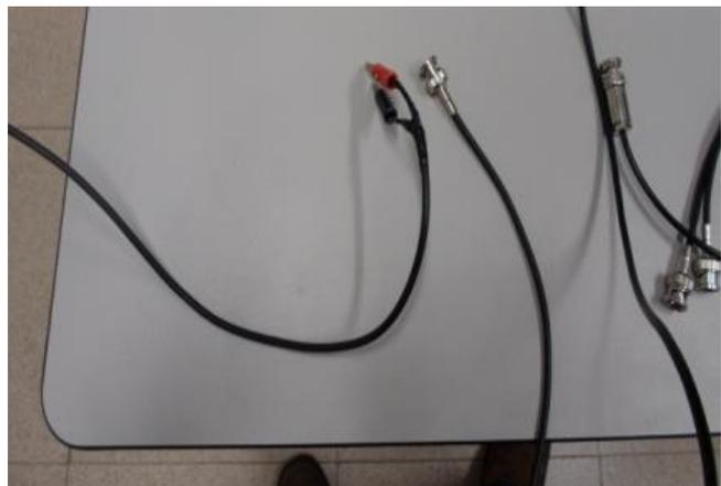
Fig.4.10 Cable adaptado de BNC a bananas
