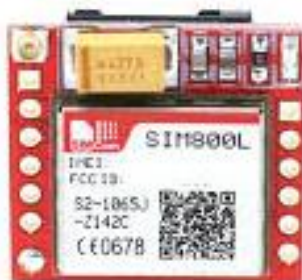
Figura 2.9 Modulo SIM800L GSM/GPRS
