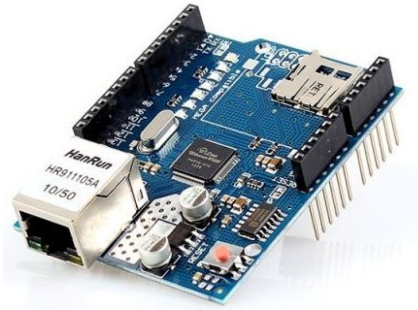
Figura 3.9: Arduino Ethernet Shield HR911105A
