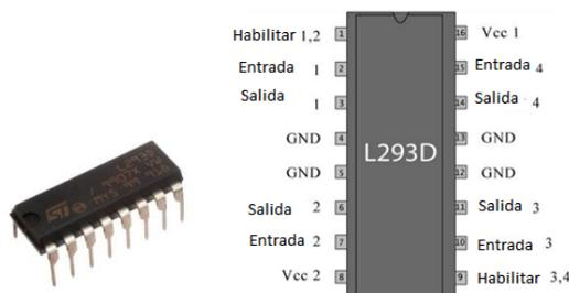
**Figura 4.1**L293D.**Figura 4.2**Pines de L293D.
