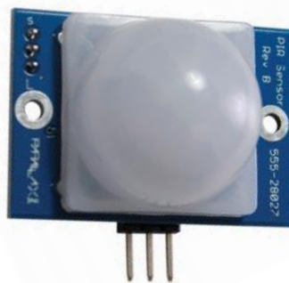
Figura 2.4 Sensor PIR (Rev B).
