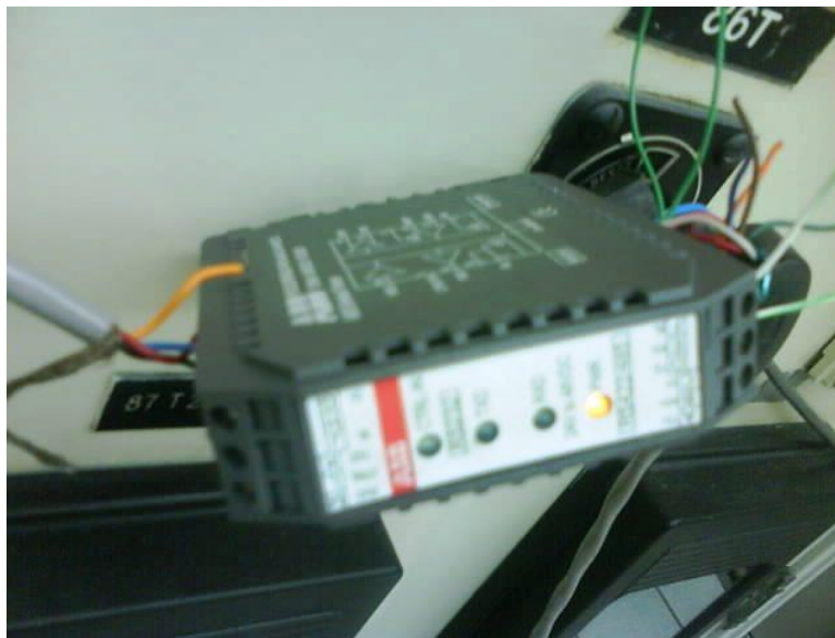
Figura 3.3.7: transceiver RS232 a RS485.
