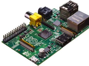
*Fig. 4.1 Raspberry pi modelos B.*
