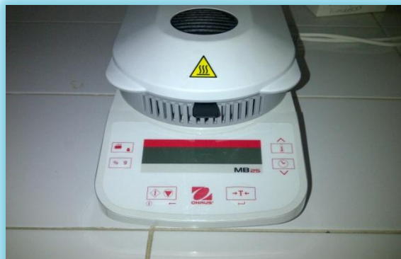
Figura No 6. MB25 Termo Balanza (OHAUS®)
