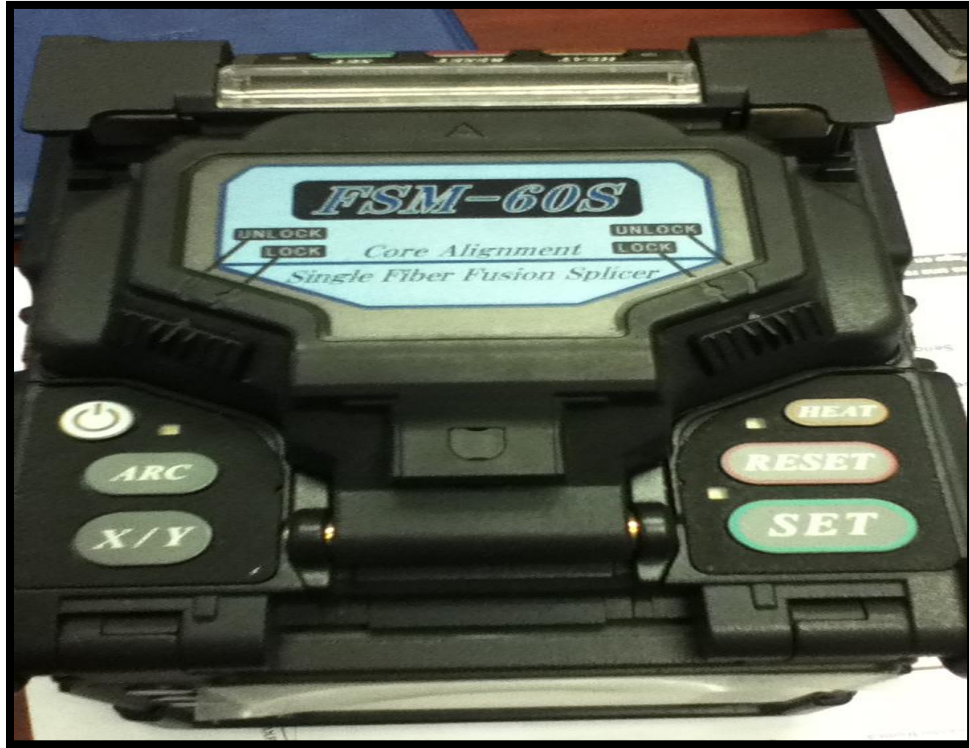
Figura 4.3 Empalmadora FUJIKURA FSM-60S.
