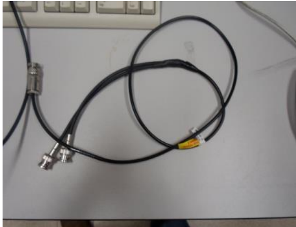
Figura III.9 Cable adaptado de triaxial a coaxial.
