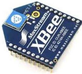
Figura 4.12 Transmisor/Receptor XBee
